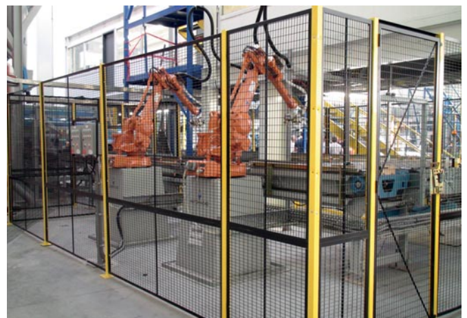
Fig. 2: Along with the robots, Automacad delivers a custom risk assessment solution which includes safety sensors and fences to guarantee your employees' safety around the robots.
