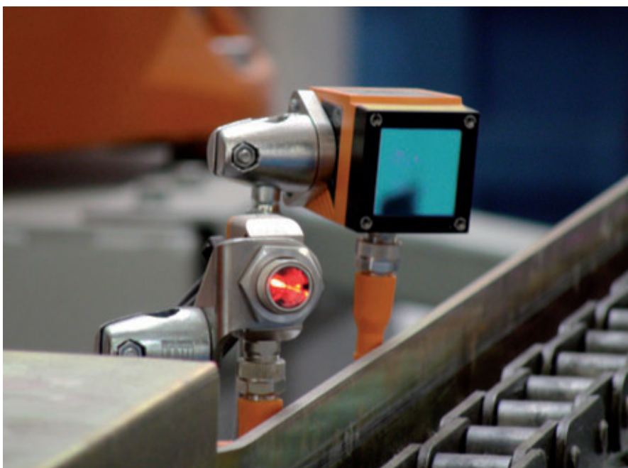
Automacad deployed sensors from ifm efector North America throughout the Stonedge plant to track product as it moves through the facility and feed information to the Automacad-designed SCADA central control system.
