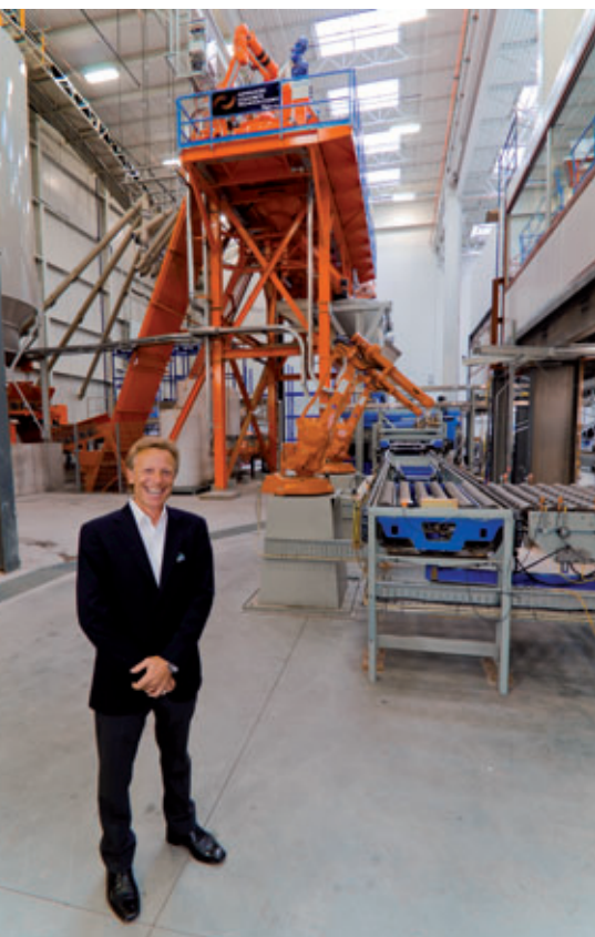
Charles Ciccarello, founder and president of Techo-Bloc, stands on the manufacturing floor of the new 80,000 sq. ft. Stonedge wet cast products plant his company recently completed in Chambly, Quebec, Canada. Just behind him is the Automacad-provided wet line (nearest) and (in orange in background) the ACT MobilMat mo2250-750 automatic concrete batching system.
