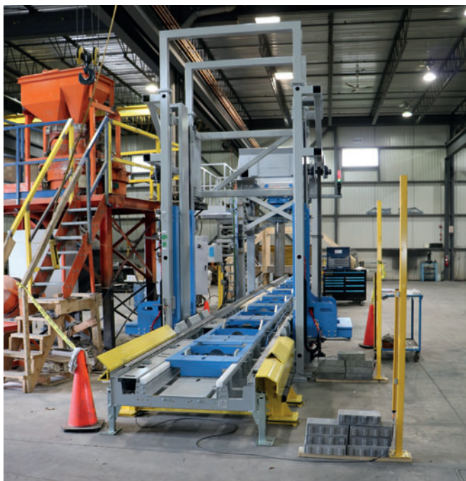
Fig 8: An automatic conveyor line runs next to a small batching system that feeds and automated filling system, leading to a curing conveyor at the far end.
