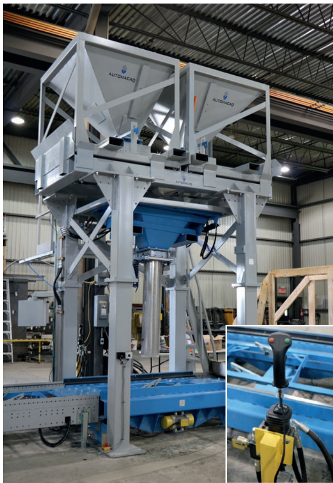
Fig. 5: Joy-stick controlled (inset) two-color filling system makes it easy to adjust and modify colors to create a variety of products.
