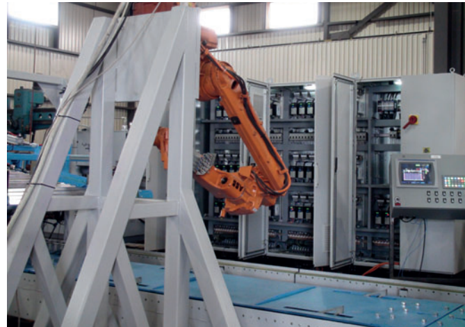
Fig. 4: Computerized control system coordinates operation of entire wet cast alternative masonry production facility. Operator control panel can be seen at right. An Automacad Color-I robotic coloration system is in orange in the park position.
