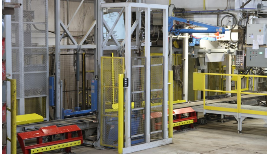
Wet line with an automatic release agent applicator
