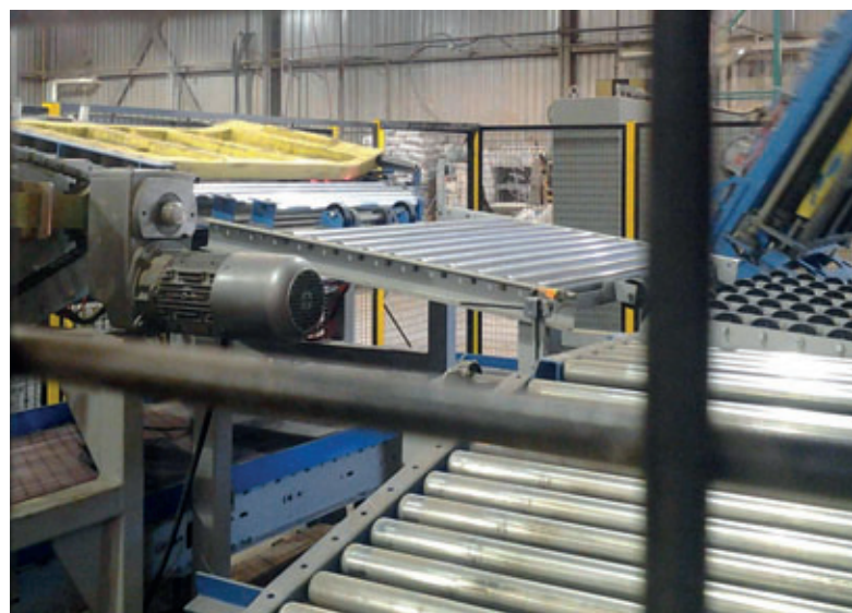
Post-demolding mold return to be rematched with a carrier
