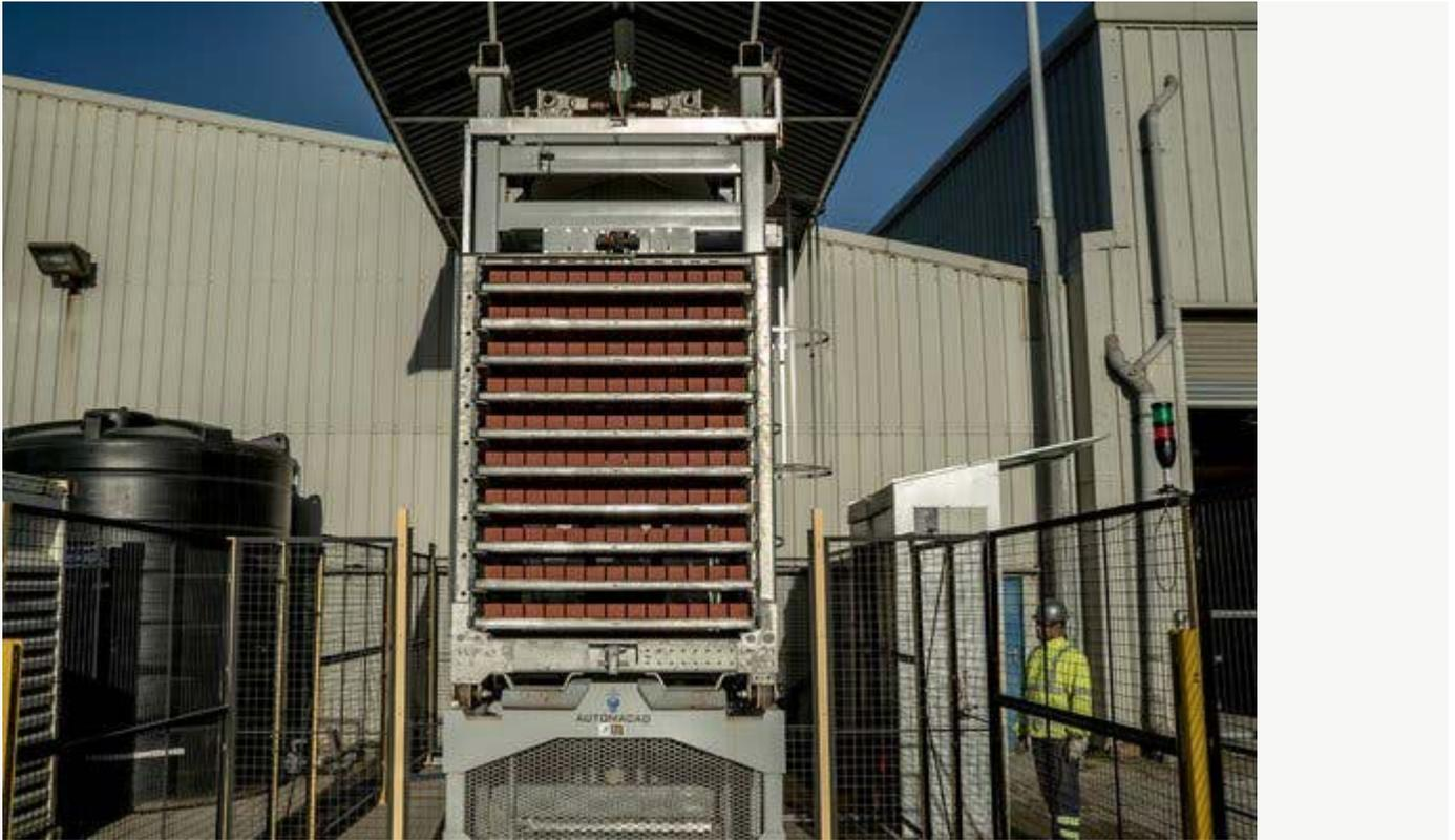
A batch of Solidia's bricks in Leighton Buzzard being readied to be sealed and infused with carbon dioxide. Credit... Andrew Testa for The New York Times
